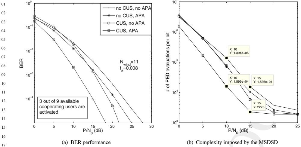
**Figure 13.12:** BER performance and the MSDSD complexity reductions achieved by the CUS and APC schemes for DAF-aided DQPSK-modulated user-cooperative cellular uplink, where three out of nine cooperating RS candidates are activated. All other system parameters are summarized in Table 13.3.
