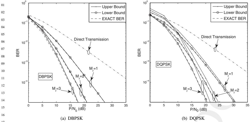
**Figure 13.3:** BER lower and upper bounds versus SNR for DAF-aided cooperative cellular systems where there are  $M_r$  activated cooperating MSs, each having fixed transmit power and location. All other system parameters are summarized in Table 13.1.
