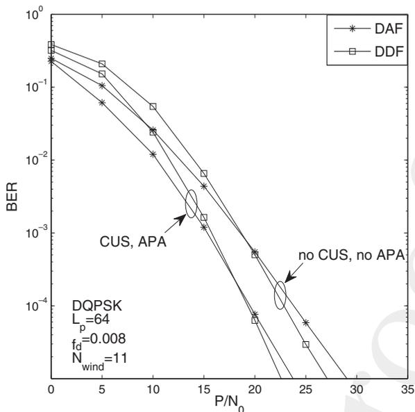
**Figure 13.19:** Performance comparison between the DAF- and DDF-aided DQPSK-modulated user-cooperative cellular systems employing the MSDSD, where two out of eight cooperating user candidates are activated. All other system parameters are summarized in Table 13.3.
