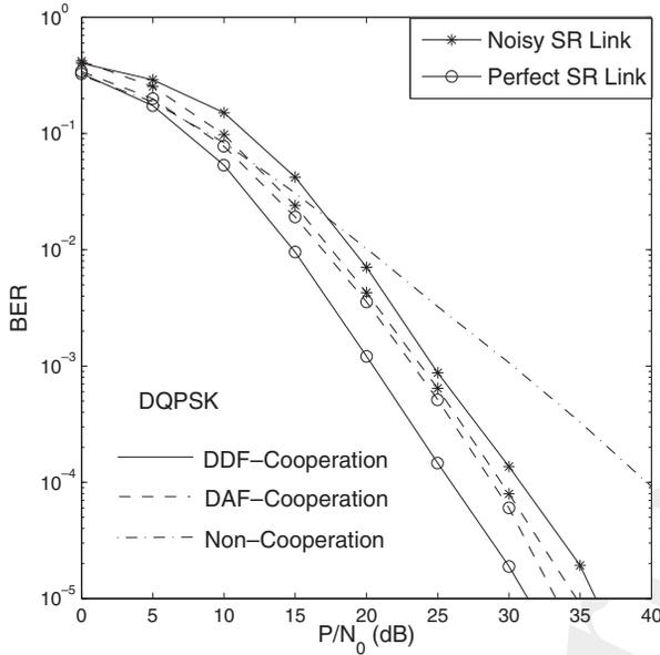
**Figure 13.18:** Impact of the source–relay link’s quality on the end-to-end BER performance of a DQPSK-modulated cooperative system employing  $M_r = 1$  cooperating RS roaming about half-way between the source MS and the BS. The CDD is employed by both the RS and the BS in a Rayleigh fading channel having a Doppler frequency of  $f_d = 0.001$ .
