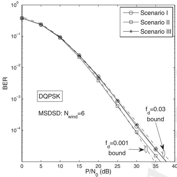
**Figure 12.19:** The impact of the relative mobility among the source, relay and destination nodes on the BER performance of the DAF-aided T-DQPSK-modulated cooperative system employing MSDSD at the destination node in Rayleigh fading channels. All other system parameters are summarized in Tables 12.5 and 12.6.
