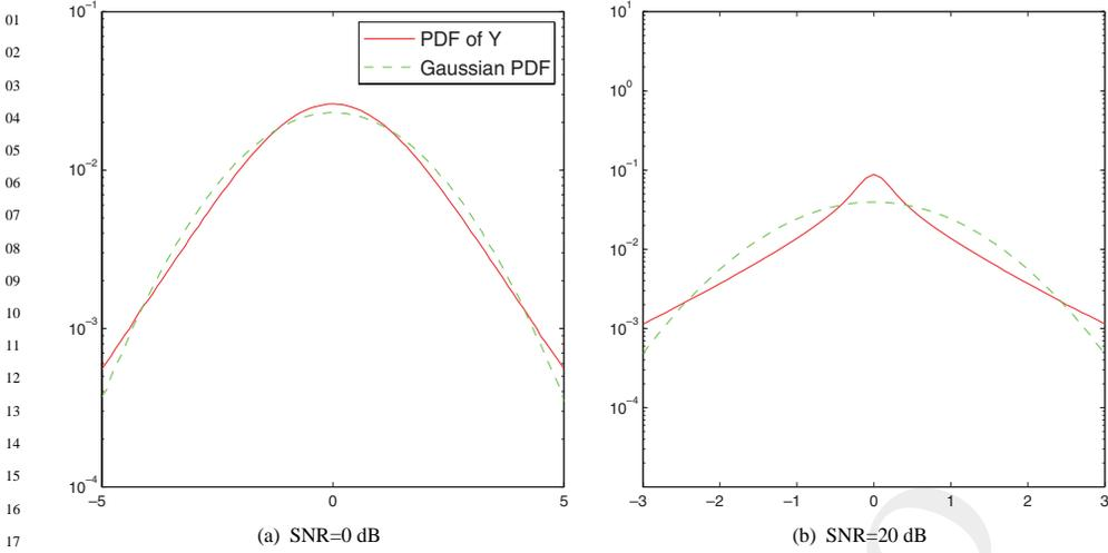
**Figure 12.16:** PDF of the received signal  $\underline{\mathbf{Y}}$  of Equation (12.64) in the DAF-aided cooperative system.
