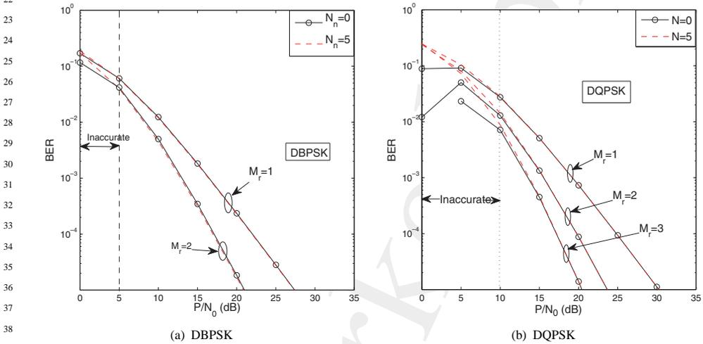
**Figure 13.4:** Impact of  $N_n$  of Equation (13.45) on the BER lower bounds versus SNR for DAF-aided cooperative cellular systems, where there are  $M_r$  activated cooperating MSs, each having fixed transmit power and location. All other system parameters are summarized in Table 13.1.
