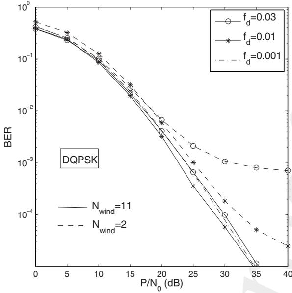
**Figure 12.18:** BER performance improvement achieved by the MSDSD scheme employing  $N_{wind} = 11$  for the DAF-aided T-DQPSK-modulated cooperative system in time-selective Rayleigh fading channels. All other system parameters are summarized in Table 12.5.
