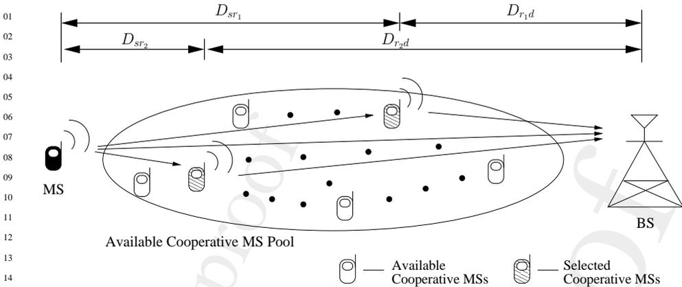
**Figure 13.1:** Cooperation-aided uplink systems using relay selection. ©IEEE Wang & Hanzo 2007 [8]
