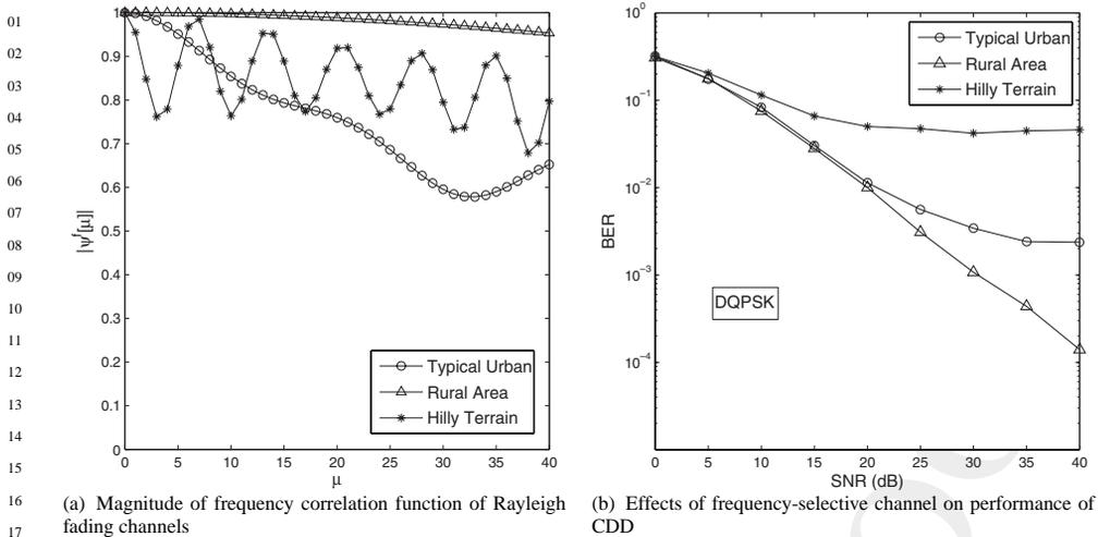
Figure 12.4: Impact of frequency-selective channels on the performance of CDD.
