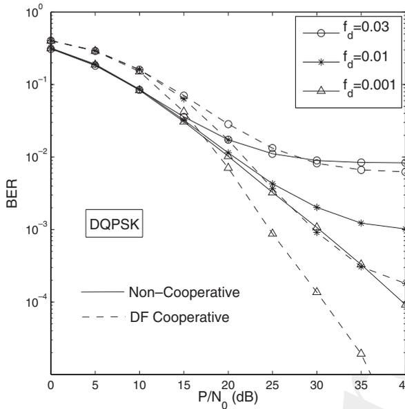
**Figure 12.12:** BER performance of the DDF-aided DQPSK-modulated cooperative system in Rayleigh fading channels at different normalized Doppler frequencies. The system parameters were summarized in Table 12.4.
