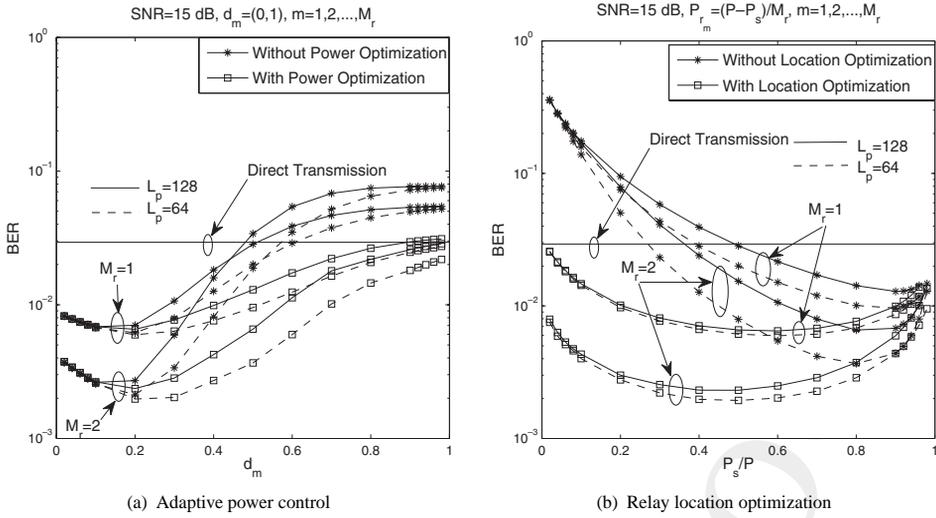
**Figure 13.14:** Power and relay location optimization for the DQPSK-modulated DDF-aided cooperative cellular systems having  $M_r$  activated cooperating MSs. All other system parameters are summarized in Table 13.4. ©IEEE Wang & Hanzo 2007 [8]
