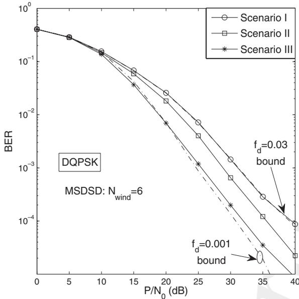
**Figure 12.23:** The impact of the relative mobility among the source, relay and destination nodes on the BER performance of the DDF-aided T-DQPSK-modulated cooperative system employing MSDSD at both the relay and destination nodes in Rayleigh fading channels. All other system parameters are summarized in Tables 12.5 and 12.6.
