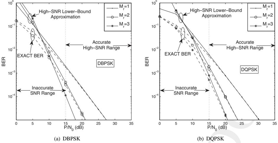
**Figure 13.5:** High-SNR-based BER lower bounds versus SNR for DAF-aided cooperative cellular systems, where there are  $M_r$  activated cooperating MSs, each having transmit power and location. All other system parameters are summarized in Table 13.1.
