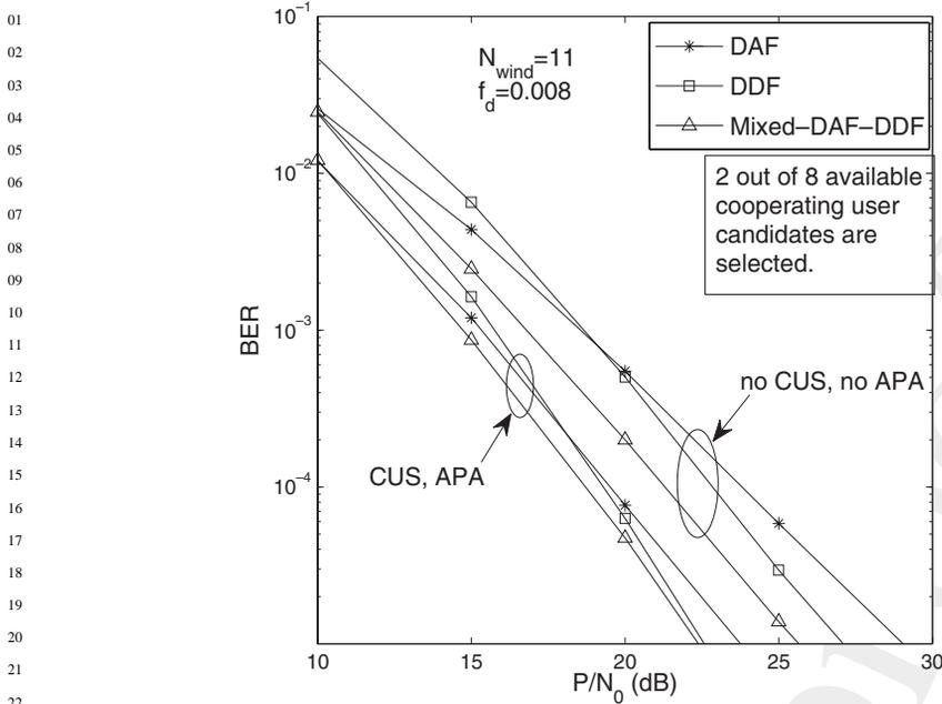
**Figure 13.21:** Performance improvement by the joint CPS and CUS for the DQPSK-modulated user-cooperative cellular uplink employing the MSDSD, where two out of eight cooperating user candidates are activated. All other system parameters are summarized in Table 13.3.
