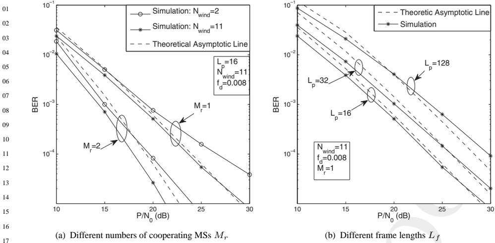
**Figure 13.6:** BER performance versus SNR for DDF-aided cooperative cellular systems, where there are  $M_r$  activated cooperating MSs, each having fixed transmit power and location. The MSDSD using  $N_{wind} = 11$  is employed at the BS. All other system parameters are summarized in Table 13.2.
