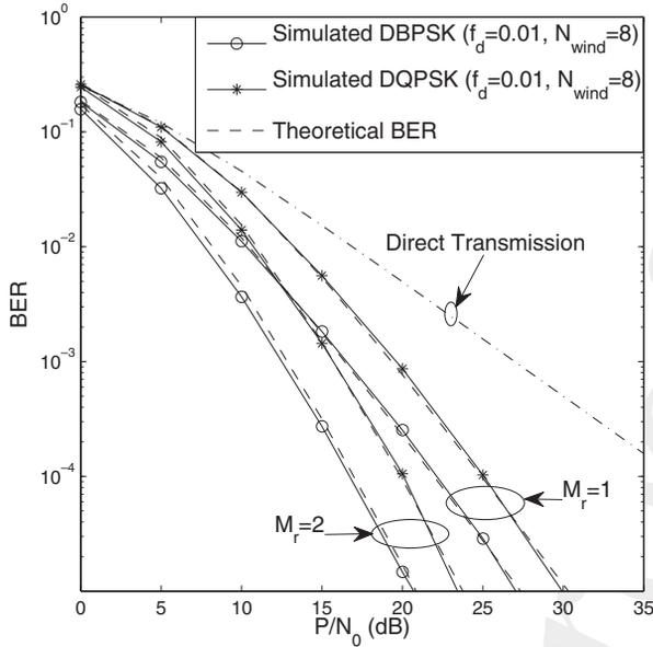
**Figure 13.2:** BER performance versus SNR for DAF-aided cooperative cellular systems, where there are  $M_r$  activated cooperating MSs, each having fixed transmit power and location. The MSDSD using  $N_{wind} = 8$  is employed at the BS. All other system parameters are summarized in Table 13.1.
