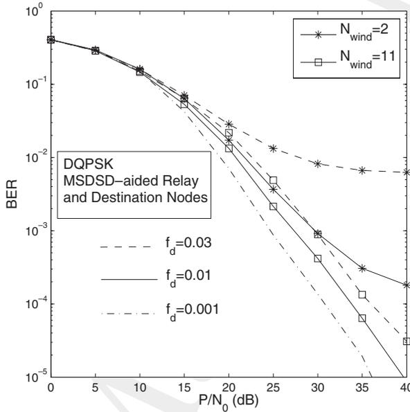
**Figure 12.21:** BER performance improvement achieved by the multi-path MSDSD employing  $N_{wind} = 11$  at the destination node of the DDF-aided T-DQPSK-modulated cooperative system in Rayleigh fading channels. All other system parameters are summarized in Table 12.5.
