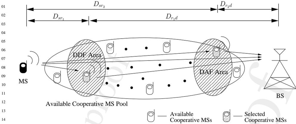
**Figure 13.20:** Cooperation-aided uplink systems using the joint CPS and CUS scheme.
