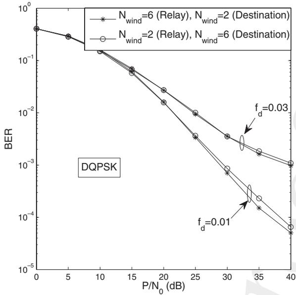
**Figure 12.22:** BER performance of the DDF-aided T-DQPSK-modulated cooperative system employing MSDSD in conjunction with different detection-complexity allocations in Rayleigh fading channels. All other system parameters are summarized in Table 12.5.
