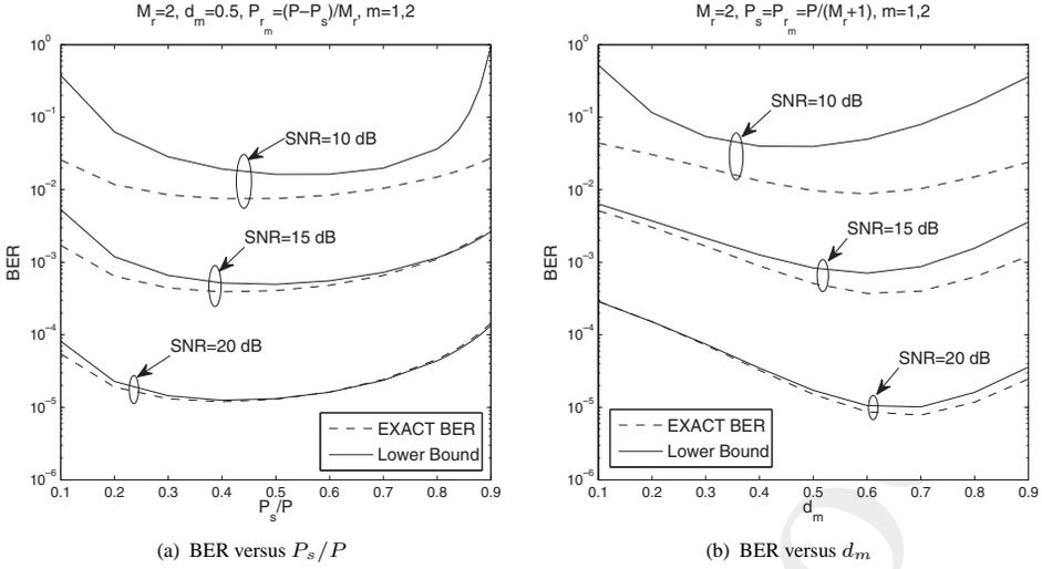
**Figure 13.8:** Effects of the SNR on the tightness of the high-SNR-based BER lower bound for the DQPSK-modulated DAF-aided cooperative cellular uplink having two activated cooperating MSs. All other system parameters are summarized in Table 13.3.
