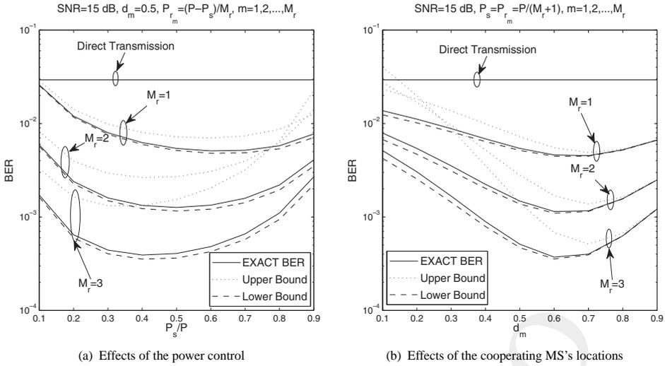
**Figure 13.7:** Effects of the power control and of the cooperating MS's location on the BER performance of DQPSK-modulated DAF-aided cooperative cellular systems having  $M_r$  activated cooperating MSs. All other system parameters are summarized in Table 13.3.
