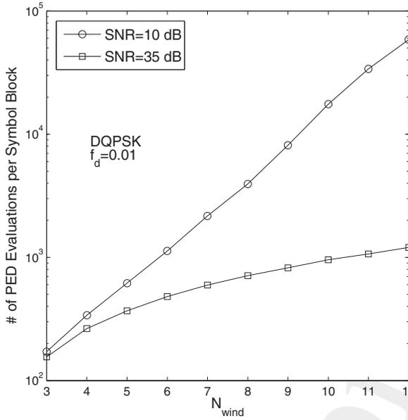
Figure 12.7: Complexity imposed by the MSDSD versus the observation window size  $N_{wind}$ .
