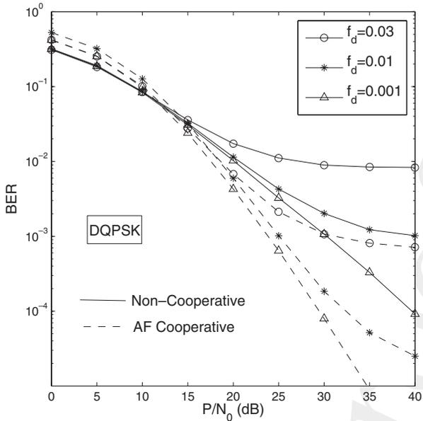
**Figure 12.11:** BER performance of the DAF-aided DQPSK-modulated two-user cooperative OFDM system in Rayleigh fading channels at different normalized Doppler frequencies. The system parameters were summarized in Table 12.4.
