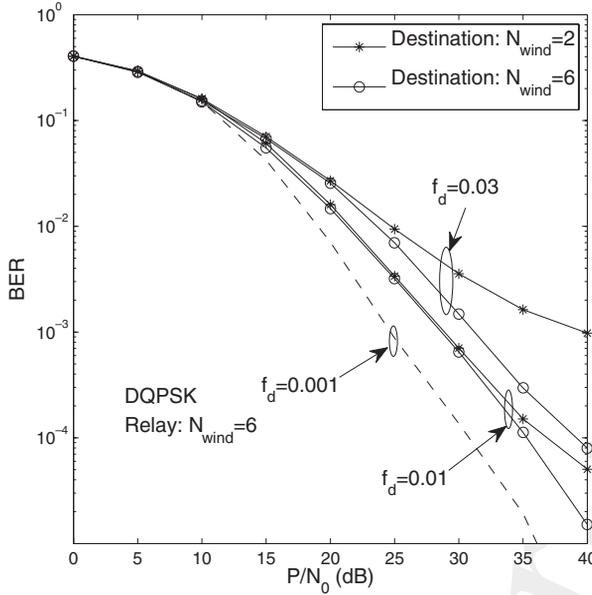
**Figure 12.20:** BER performance improvement achieved by the multi-path-based MSDSD scheme employing  $N_{wind} = 6$  at the destination node of the DDF-aided T-DQPSK-modulated cooperative system in Rayleigh fading channels. All other system parameters are summarized in Table 12.5.
