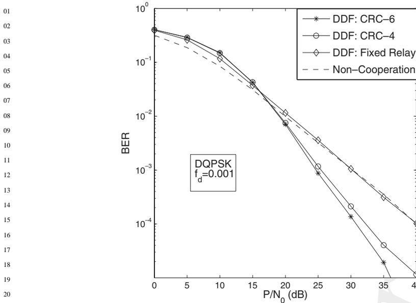
**Figure 12.13:** Benefits of the CRC-based error-detection capability at the relay node on the end-to-end BER performance of a DDF-aided DQPSK-modulated cooperative system. The system parameters were summarized in Table 12.4.
