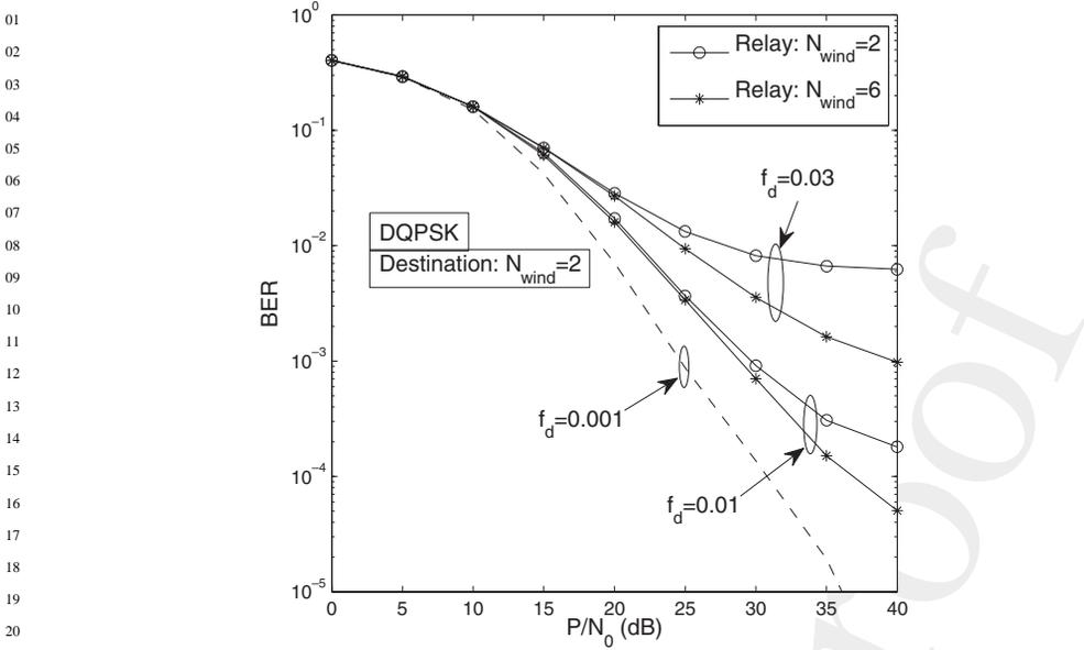
**Figure 12.15:** BER performance of DDF-aided DQPSK-modulated cooperative system using MSDSD-aided relays in Rayleigh fading channels.
