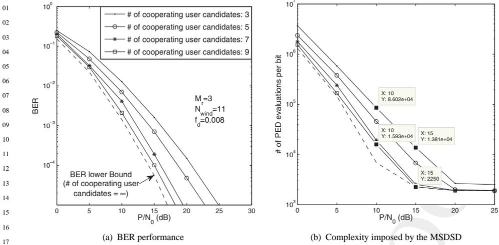
**Figure 13.13:** The effects of the size of the cooperating RS pool on the DAF-aided DQPSK-modulated user-cooperative cellular uplink employing the CUS and APC schemes, where  $M_r = 3$  cooperating users are activated. All other system parameters are summarized in Table 13.3.
