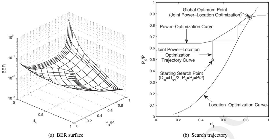
**Figure 13.10:** Optimum cooperative resource allocation for DQPSK-modulated DAF-aided cooperative cellular systems having a single activated cooperating MS at SNR = 15 dB. All other system parameters are summarized in Table 13.3.
