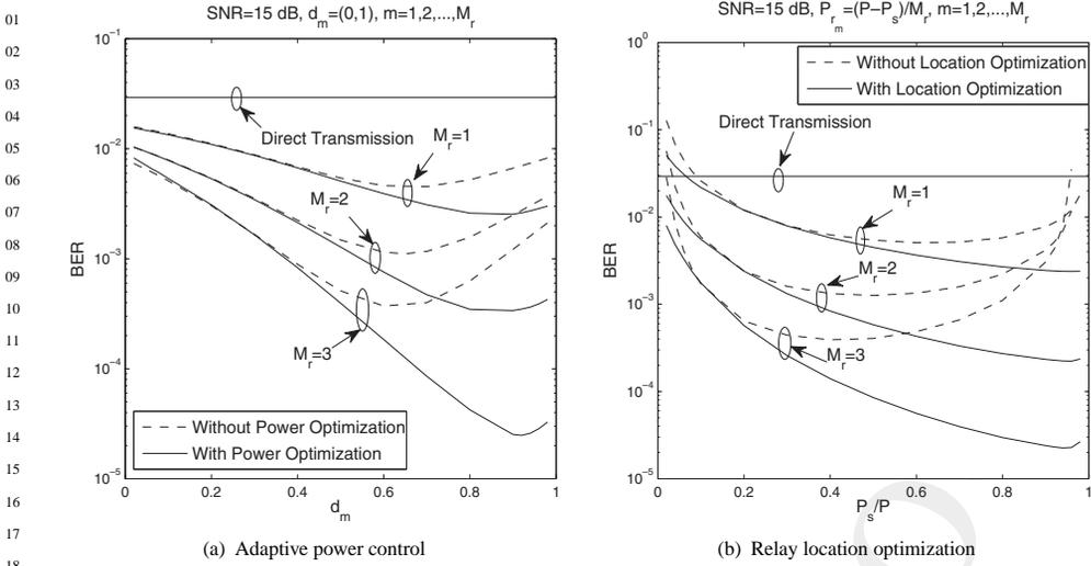
**Figure 13.9:** Power and relay location optimization for DQPSK-modulated DAF-aided cooperative cellular systems having  $M_r$  activated cooperating MSs. All other system parameters are summarized in Table 13.3. ©IEEE Wang & Hanzo 2007 [8]
