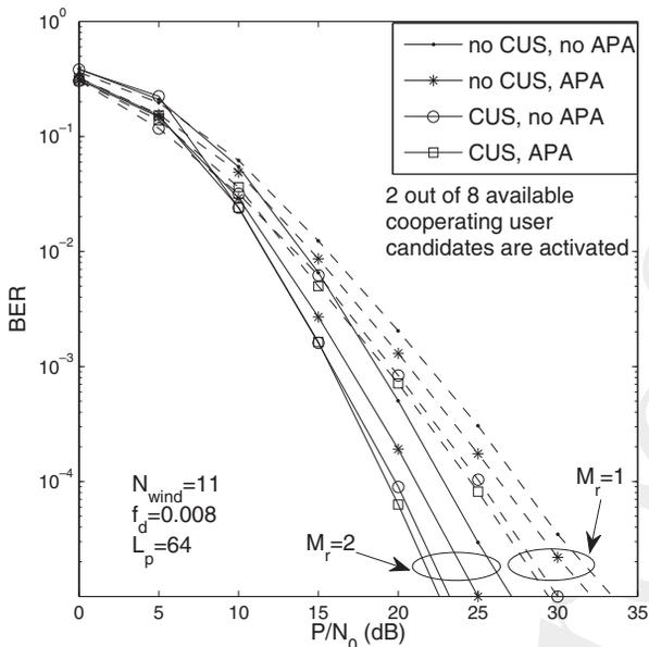
**Figure 13.17:** Performance improvements achieved by the CUS and APC schemes for the DDF-aided DQPSK-modulated user-cooperative cellular system employing the MSDSD in a relatively fast Rayleigh fading channel, where two out of eight cooperating users are activated. All other system parameters are summarized in Table 13.4.
