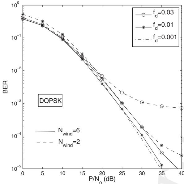
**Figure 12.17:** BER performance improvement achieved by the MSDSD employing  $N_{wind} = 6$  for the DAF-aided T-DQPSK-modulated cooperative system in time-selective Rayleigh fading channels. All other system parameters are summarized in Table 12.5.
