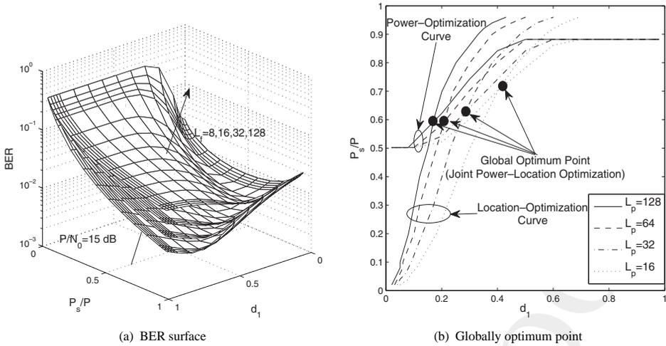
**Figure 13.15:** Optimum cooperative resource allocation for the DQPSK-modulated DDF-aided cooperative cellular systems having a single activated cooperating MS at SNR = 15 dB. All other system parameters are summarized in Table 13.4.
