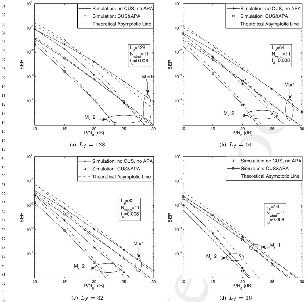
**Figure 13.16:** Performance improvement achieved by optimizing the cooperative resources for the DQPSK-modulated DDF-aided cooperative cellular systems employing the MSDSD in a relatively fast Rayleigh fading channel, where the  $M_r$  activated cooperating users are assumed to be situated at their optimum location. All other system parameters are summarized in Table 13.4.
